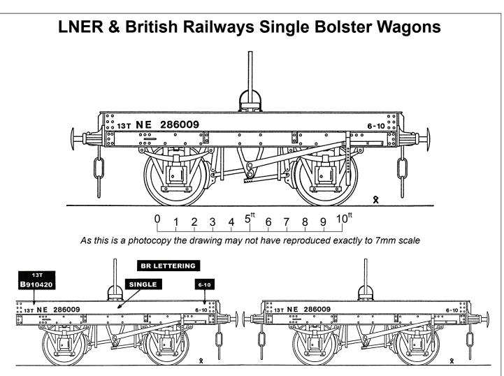
**LNER Livery.** Bodywork - Grey (RailMatch paints LNER freight grey No 624). Solebars, running gear and buffers - black. Dirty wood floor planks. Steelwork on bolsters should be grey in theory but would probably be dirty and rusty in practice. White lettering and white end of brake lever.
