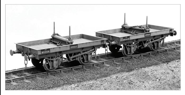
**PROTOTYPE.** These were the last design of 13 ton single bolster wagon built by the LNER between 1945 and 1948. The design was continued by British Railways who built 8000 between 1949 and 1957 as a BR standard wagon. They continued in revenue earning service until 1972 and remained in engineers use and in internal user fleets at docks and steelworks etc into the 1980's.
