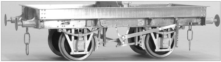
**Parts 8, Vee Hangers**. Fold up and solder to underside of floor, (note etched marks to help position).
